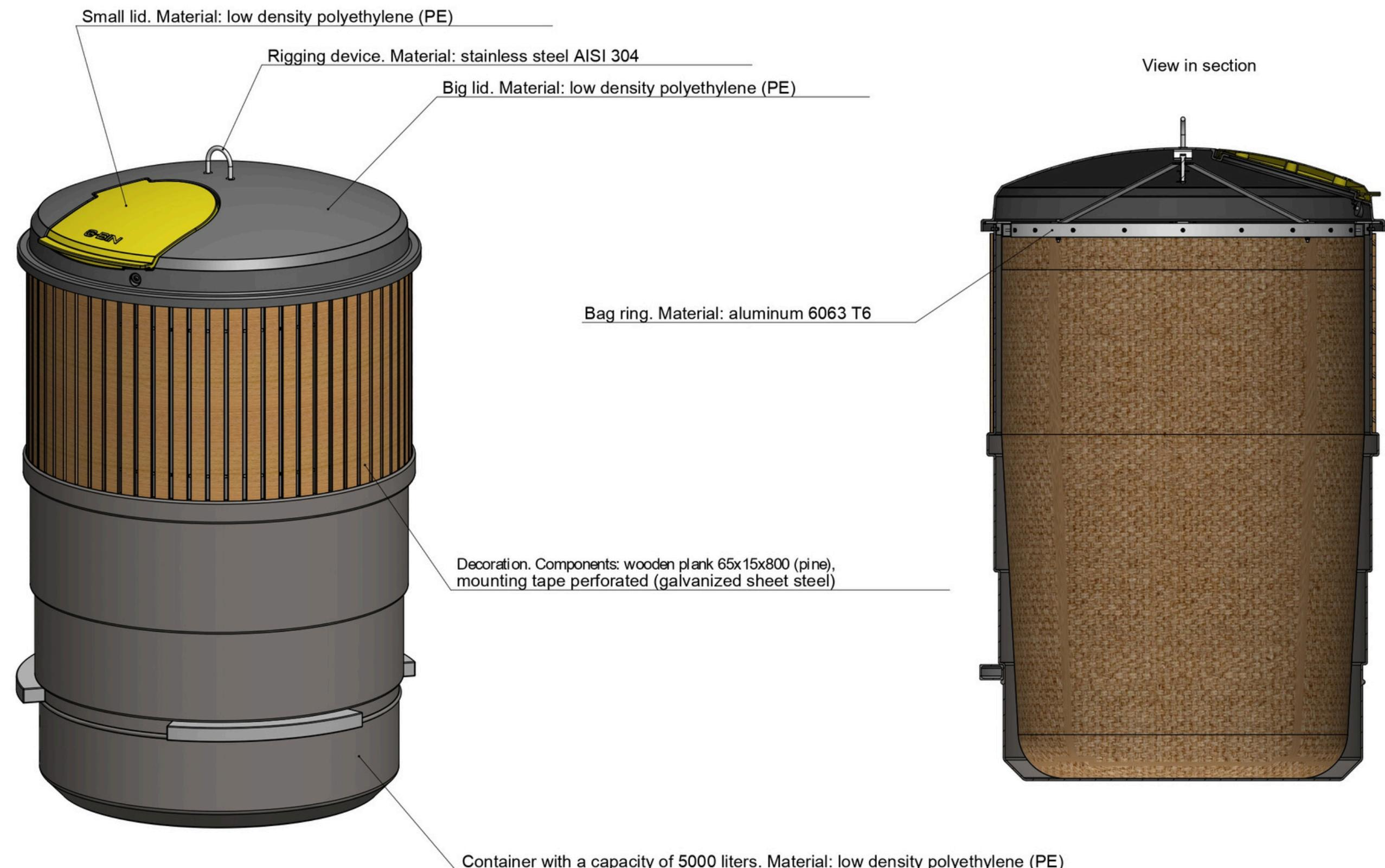
**Semi-underground waste container with a capacity of 5,000 l**
